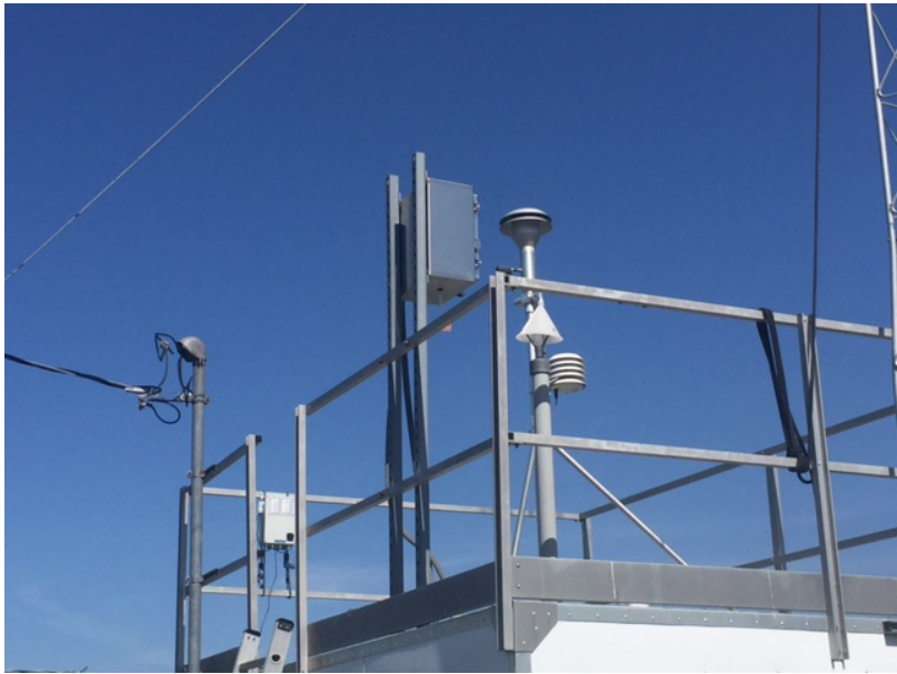
Quapaw Criteria Pollutant Shelter Site with Aeroqual sensor evaluation.
