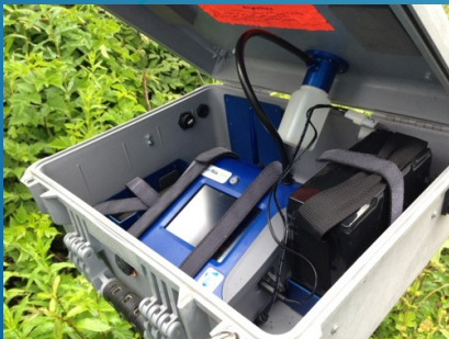
Outdoor Road Dust Monitoring Equipment Setup from the ANTHC.
